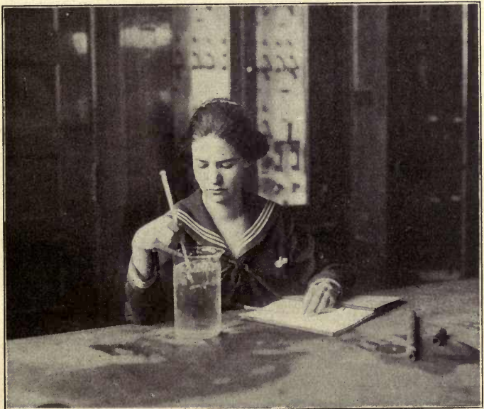
TAKING THE TEMPERATURE OF MELTING ICE TO DETERMINE THE MELTING OR FREEZING POINT.
